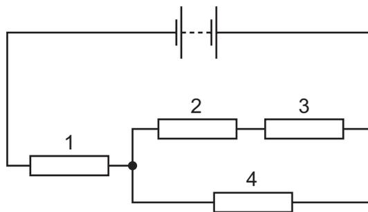
In which resistor does the current have the largest value?
